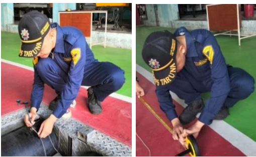
Fig 14. Roller Circumference Measurement
