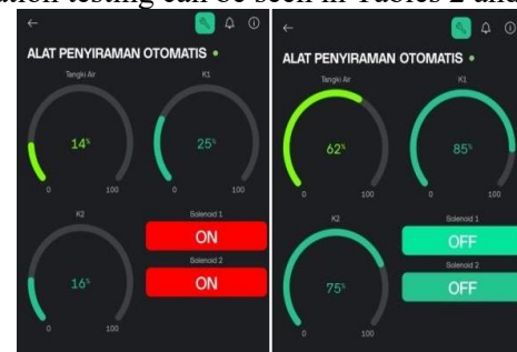
Fig. 6 Blynk App Display When Solenoid is ON and OFF
